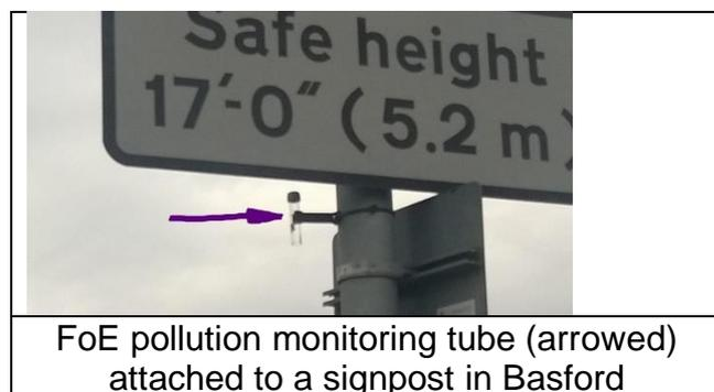
FoE pollution monitoring tube (arrowed) attached to a signpost in Basford
